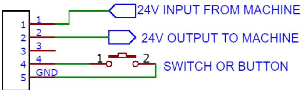
Please note that a switch/button needs to be connected between the input and ground (GND).
